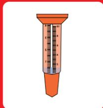
A **rain gauge** is used to measure the amount of rain that has fallen over a period of time. The tipping bucket rain gauge was invented by Christopher Wren and Robert Hooke.
