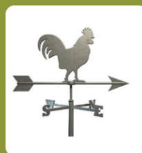
A **wind vane** is an instrument that is used to measure the direction of the wind. The Greek astronomer Andronicus invented the first weather vane. The wind vane is also known as a weather vane.
